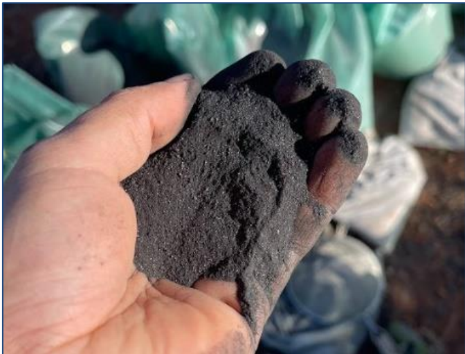
Drill Hole URC022, 5m @ 19.2% TiO 2 , 0.86g/t PGE3, 0.26% Cu, 0.78% V 2 O 5 from 12m
