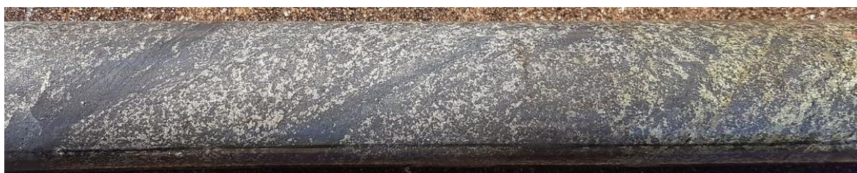
Plate 1 Example of sulphide-rich magnetite rock from hole 18CB058 (core length approx. 15 cm). Bright speckle is a combination of copper and iron sulphide. Black is magnetite.
