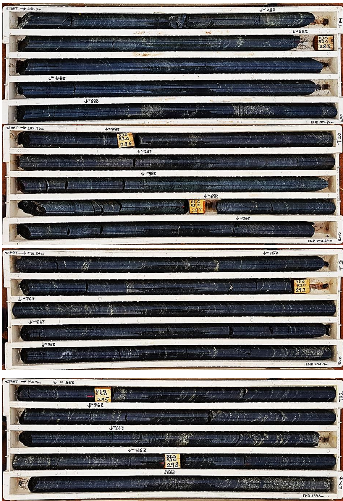
Plate 2 Example of the style of mineralisation encountered in intersections from the North Zone. This example is from hole 18CB057: 268 -299m. Black rock is magnetite. Fine yellow-bronze speckle and stripes throughout the rock is a predominantly chalcopyrite
