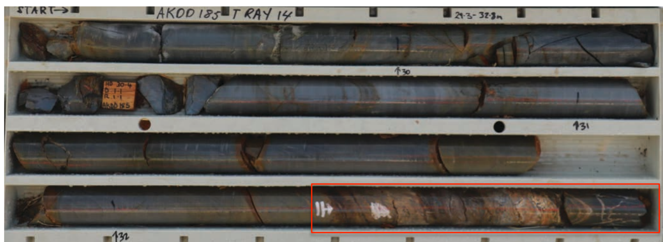
Figure 9 – AKDD185 drill core showing where 0.7m @ 5.1 g/t from 32.3m was intersected, and hosted within a narrow barite/quartz vein and alteration zone
