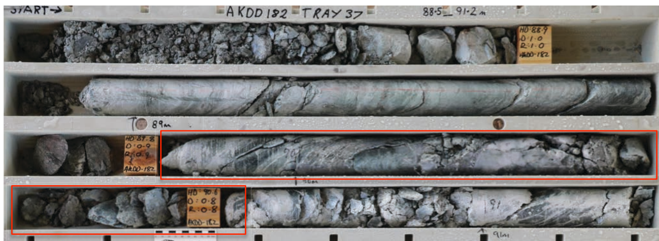
Figure 11 – AKDD182 drill core including intersection of 0.6m @ 0.8 % Cu, 44 g/t Ag and 0.8 g/t Au from 89.9m
