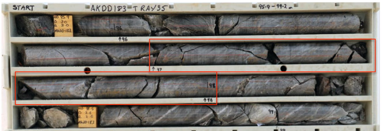
Figure 5 – AKDD183 core including intersection of 1m @ 2.3% Zn, 5.8% Zn (8.1% Pb+Zn), 41 g/t Ag and 0.2 g/t Au from 97.0m
