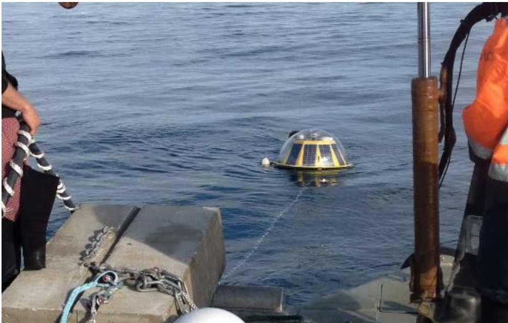
Wave measurement buoy being deployed in the CETO 6 project area
