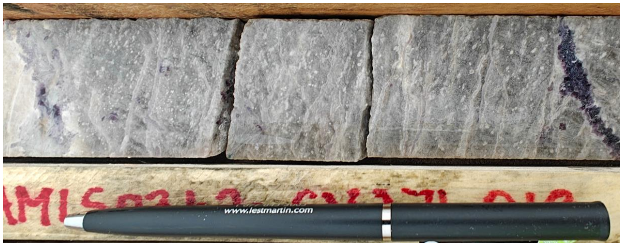
Figure 1: Pollucite mineralization in high-grade caesium drill intersection at ~64.5 m depth in drill hole CV23-271 at the Rigel Zone, CV13 Pegmatite. Interval grades 2 22.69% \text{Cs}_2\text{O} over 1.0 m (64.0 m to 65.0 m) with XRD-Rietveld reporting a pollucite content over the interval of 58%.
