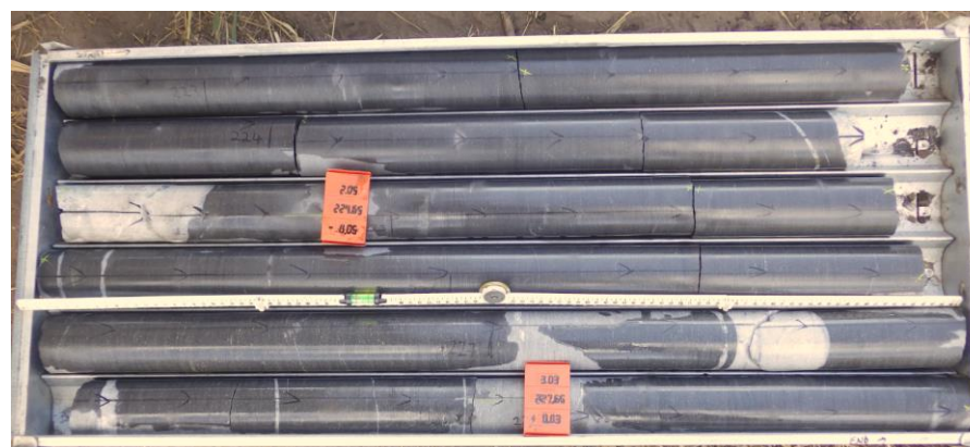
Image 12. Drill core from Nicanda Hill in Diamond Hole (GBND0001) taken from about 223m to 228m.
