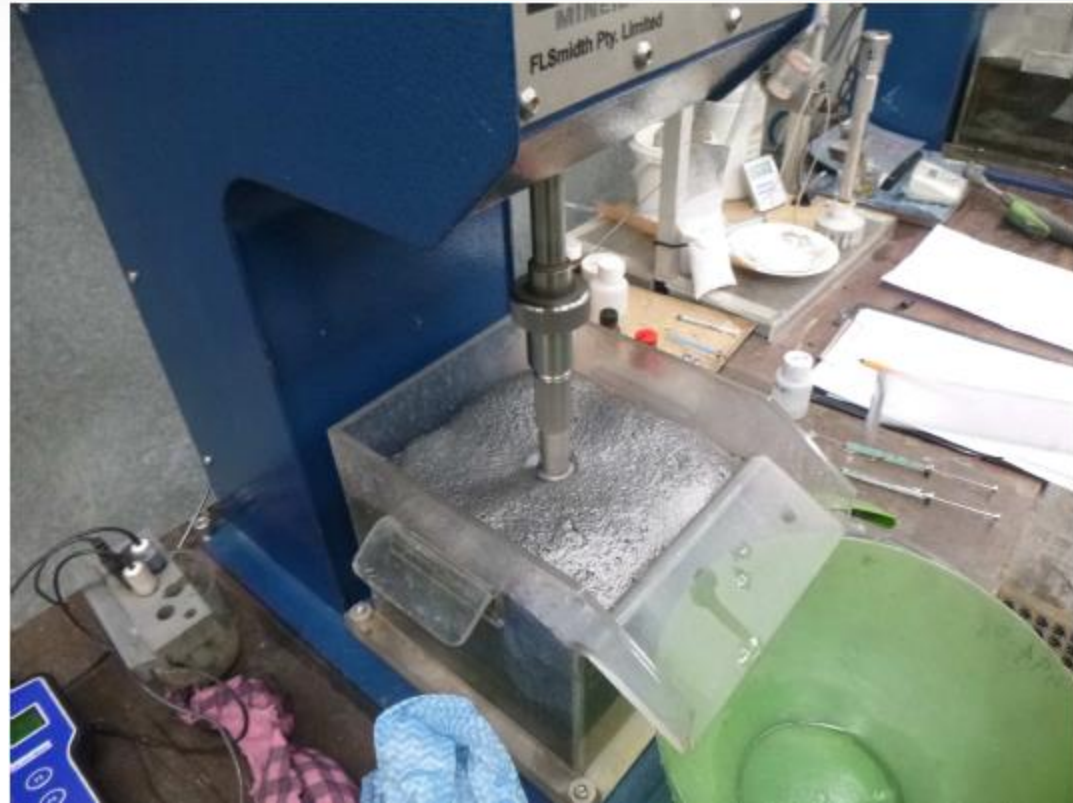
Image of the graphitic material being liberated using a flotation method at the ALS Metallurgy laboratory.
