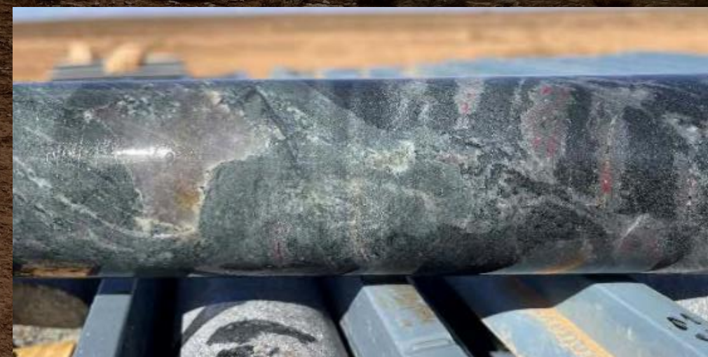
Initial first pass observation of stage 2 hydrothermal alteration of host rocks. Initial observations indicate epidotechlorite-sericite +/- actinolite and biotite alteration. Diamond HQ drill core Central_DDHC003.
