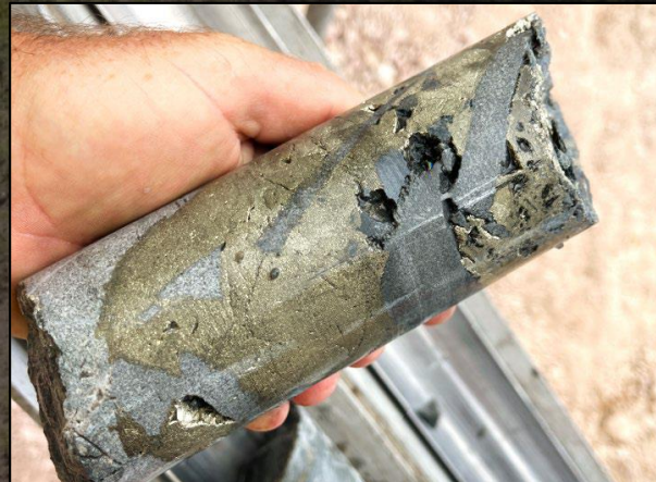
Sulfide-rich breccias from its second diamond drill hole (MPD003) contains massive sulfides infilling the metasedimentary breccia fragments. All core is HQ3 diameter. Depth of sample is approximately 110m down hole.
