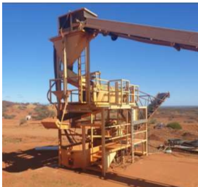
Figure 1: Fully operational 25-30tph “wash plant” acquired as part of the acquisition of M59/358
