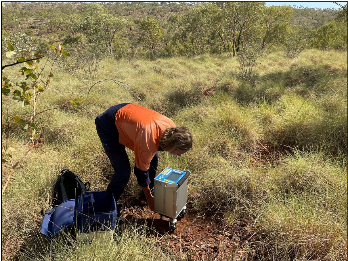
Figure 5 – Fender Geophysics team member collecting a gravity measurement
