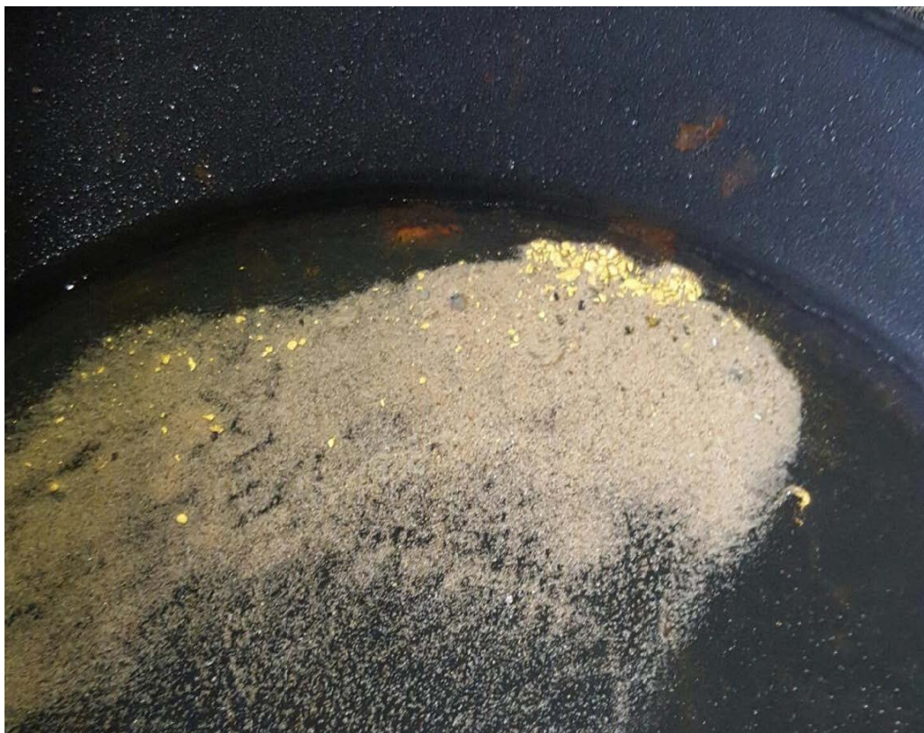
Figure 6: Gold and Sulphides from Coarse Sand Dam
