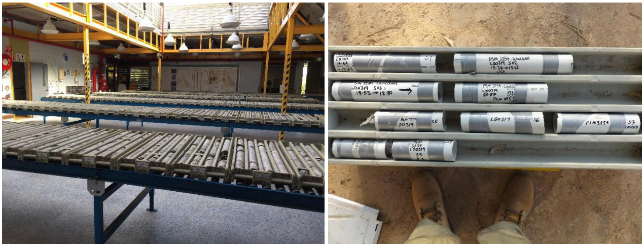
Figure 3: Left: Geotechnical drillholes laid out for scanning at the HyLogger facility in Brisbane. Right: Geotechnical samples prepared for dispatch. These are tested for mechanical strength, thus require special preparation, involving multiple layers of containment and wrapping, to avoid sustaining fractures during transport.
