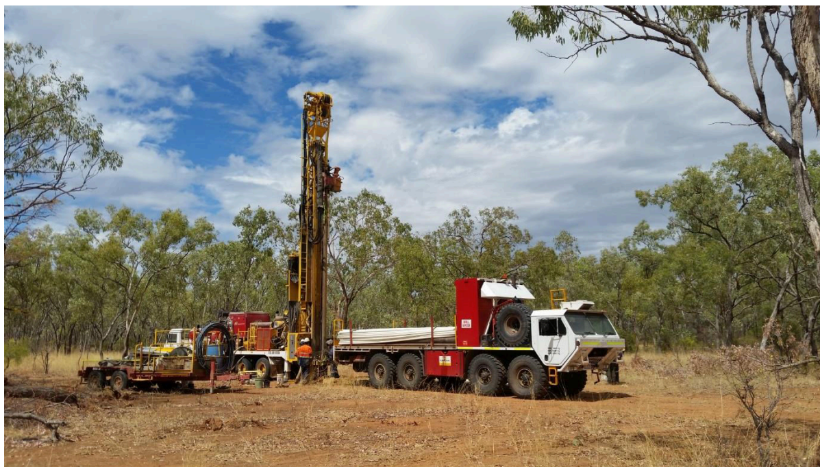
Figure 6: Groundwater monitoring bore drilling in the Lower Camp. These bores are designed to be too small to extract from and are only used to sample the quality of water for baseline environmental purposes.
