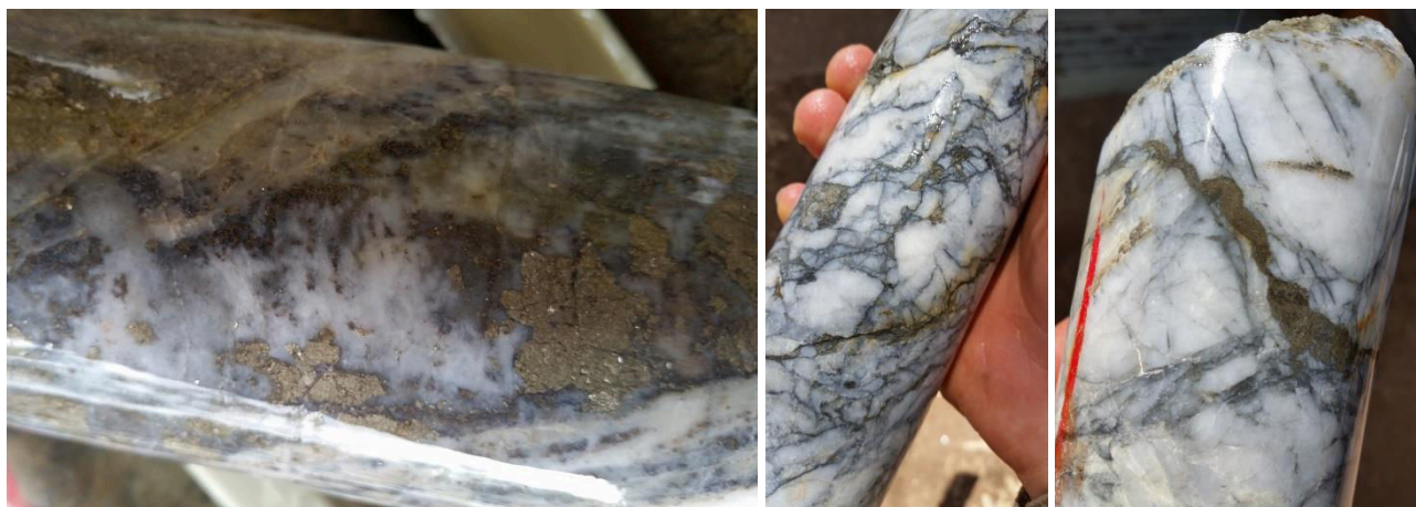
Figure 2: Example of high and moderate grade mineralisation. Left: High-grade comb quartz-sulphide (pyrite-galena-sphalerite) cavity-fill and related comb quartz-sulphide veins in recrystallised buck quartz and altered wallrock. Middle: Moderate-grade sulphidic stylo-breccia and spider quartz veinlets in recrystallised buck quartz host. Right: Shattered buck quartz with sulphide stylolite and spider quartz veinlets. Diamond drill hole LD0317. Assays pending.
