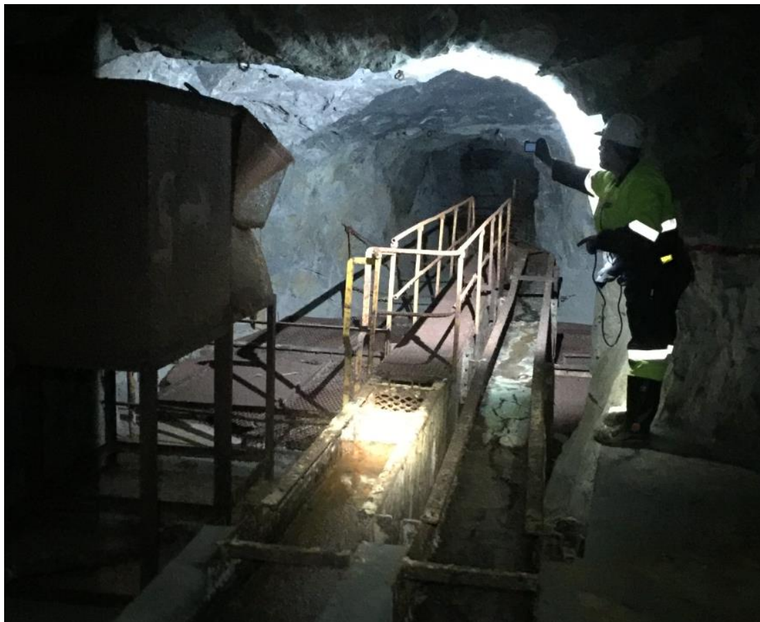
Figure 3: 294m below surface Level - Water settlers still useable.
