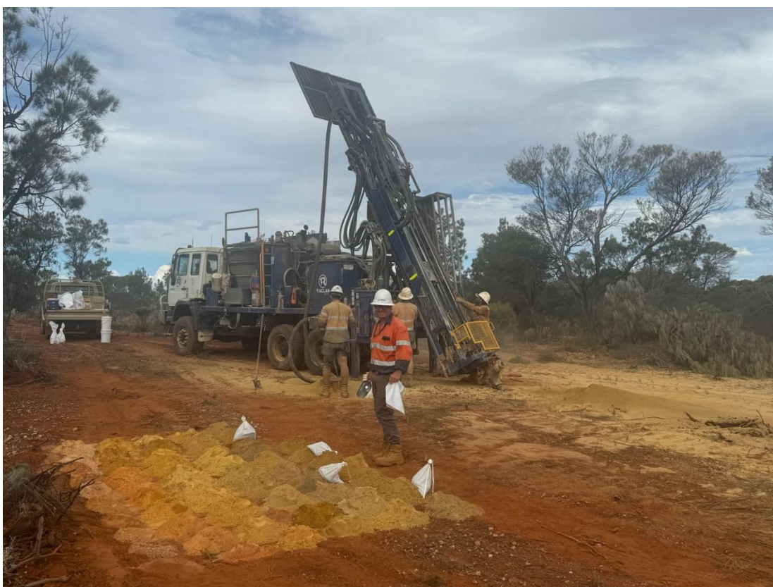
Figure 1: Aircore drilling rig Mulgabbie North
