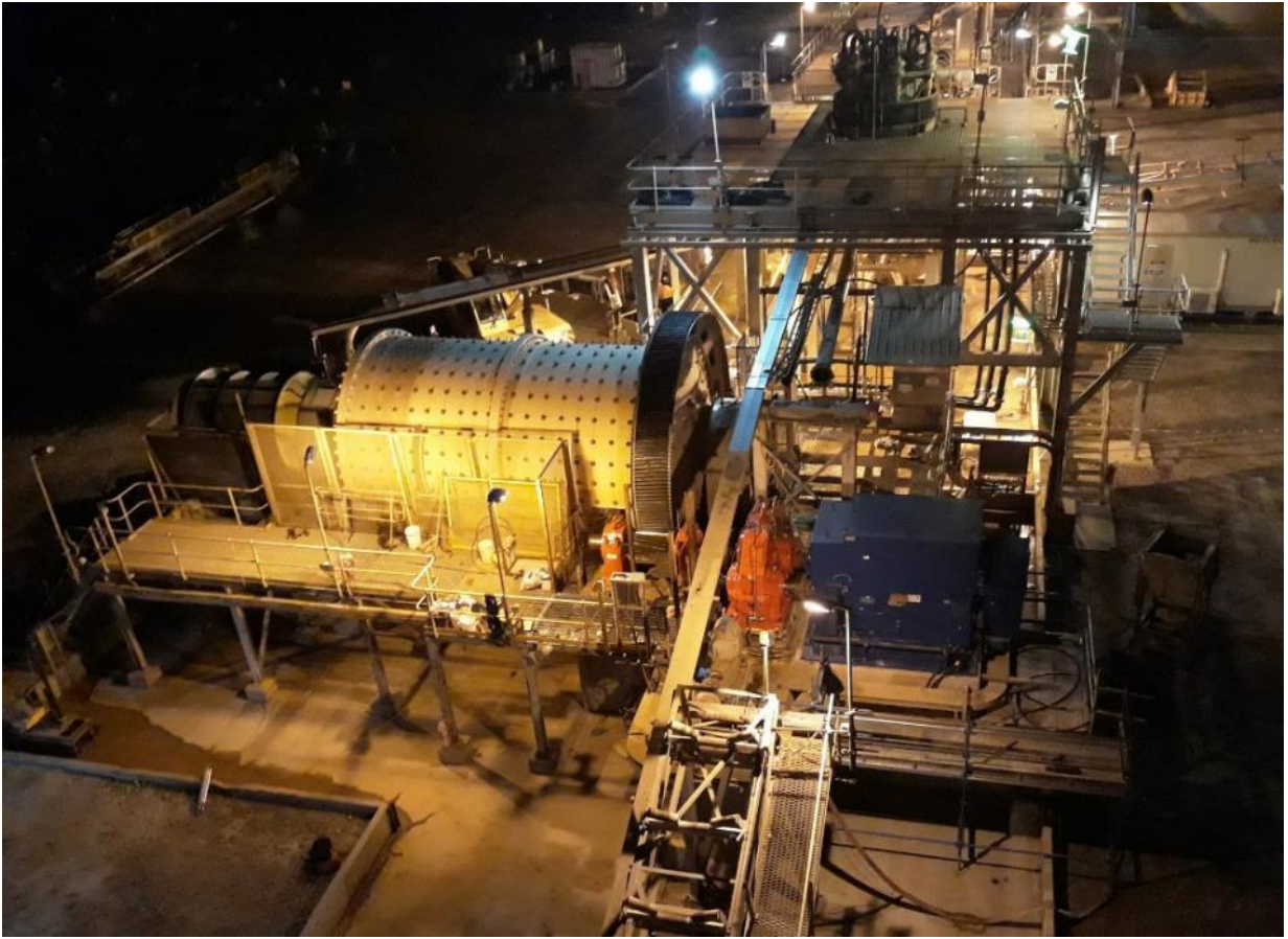
Figure A13: Existing 1800kW Ball Mill
