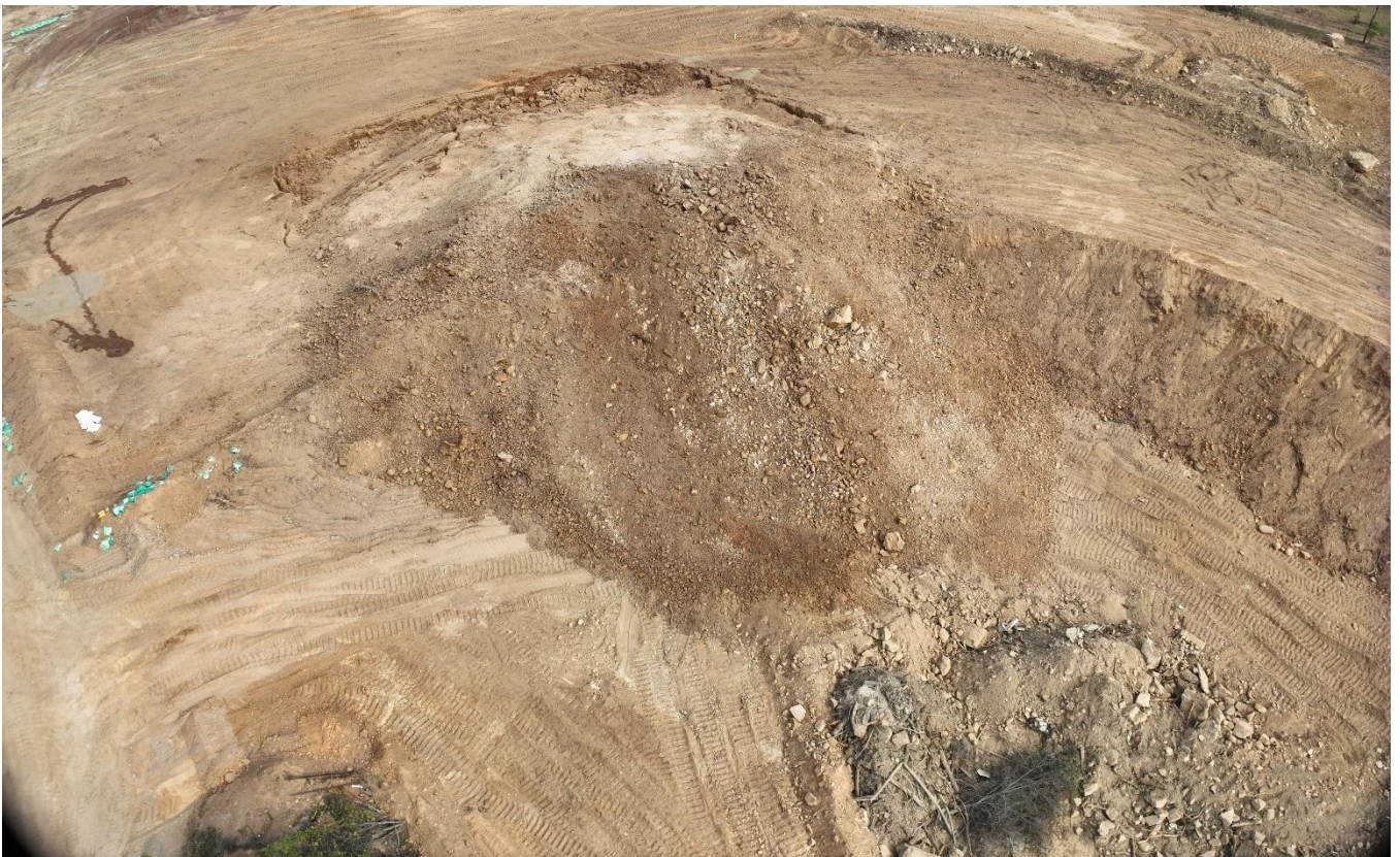
Figure 3: Close-up aerial image of the post-blast muck pile in the Southern Starter Pit at Blackjack.
