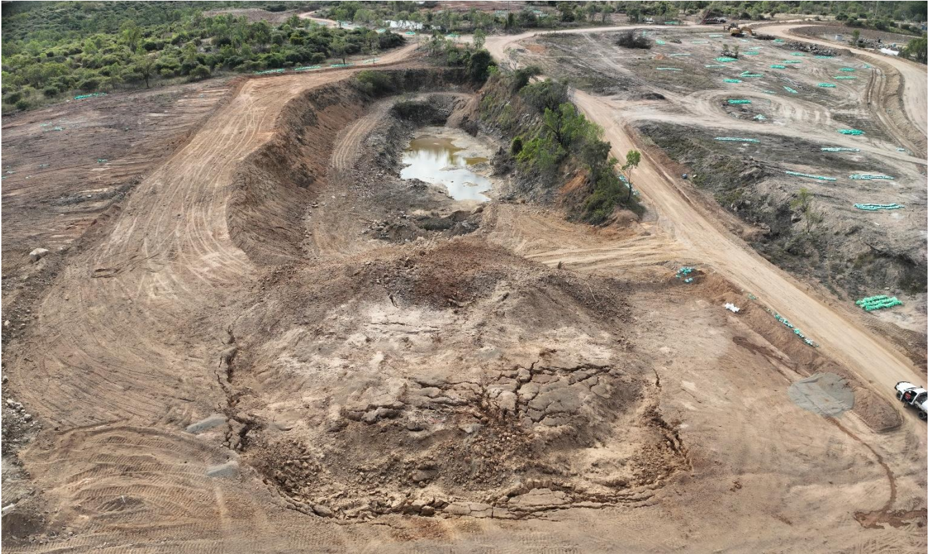
Figure 4: Post-blast aerial view of the Southern Starter Pit at Blackjack following the successful first production blast on 26 June 2025. The fractured surface and displacement of material indicate effective fragmentation, with material now ready for excavation and haulage to the ROM pad.
