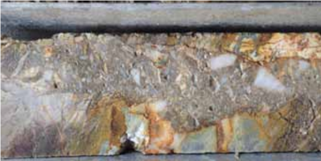
Figure 14: Hole SBDD011 (depth not noted) at Salu Bulu showing significant core axis parallel (steep) breccia zone.
