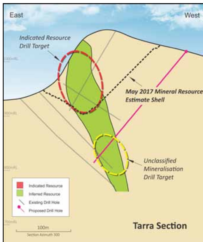
Figure 10: East-West stylised section through Tarra deposit.
