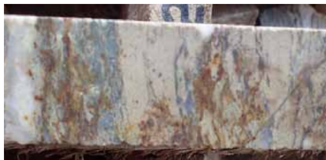
Figure 9: Photo of core from hole AMD142, approximately 65m downhole depth, showing foliation conformable type mineralisation, showing strong albite-silicate-pyrite alteration. (Willson, 2017)
