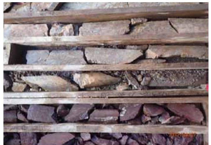
Figure 17: Sharp faulted contact between footwall hematitic mudstone and albite, silica, sericite altered hydrothermal breccia at approximately 92m downhole depth, TRD003.
