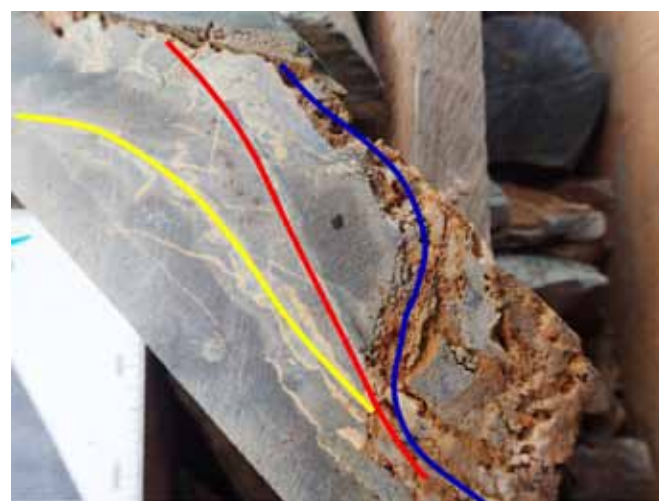
Figure 12: Veins formed under progressive deformation in hole AMD235 at approximately 14m depth. Blue – early, yellow-mid, red-late (Willson, 2017).
