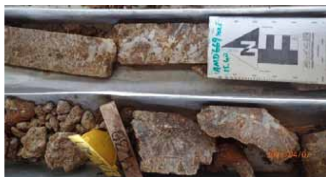
Figure 11: Semi-conformable brecciation in hole AMD669 at approximately 15.6m downhole depth with anastomosing quartz veins at a high angle to the core axis. (Willson, 2017)
