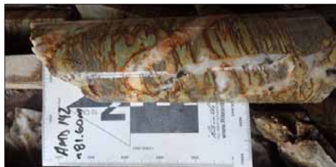
Figure 8: Core Photo – Steeply dipping mineralisation from drill hole AMD142 (81.6m down hole depth)
