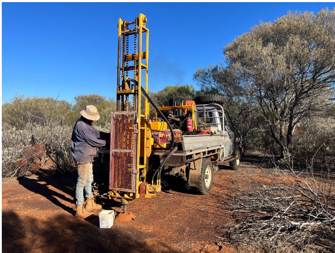
Figure 2: Auger Drilling
