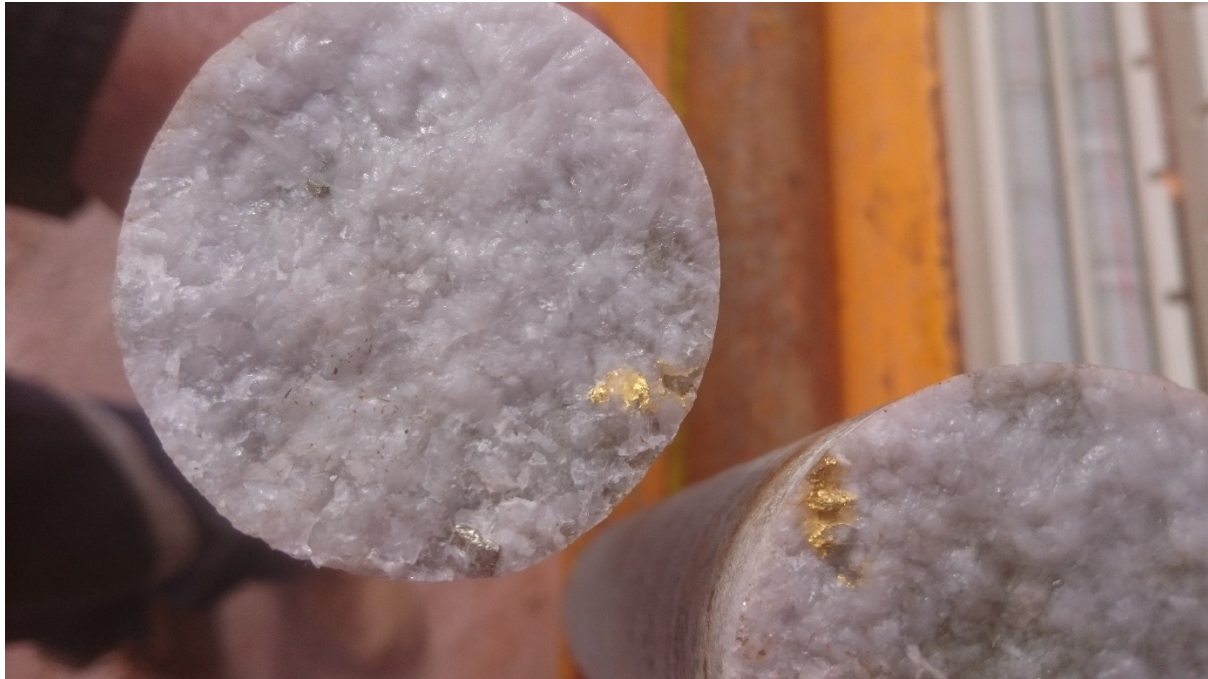
Figure 2 Coarse gold hosted by quartz veining within tonalite in MSDD264 (230.88m depth)
