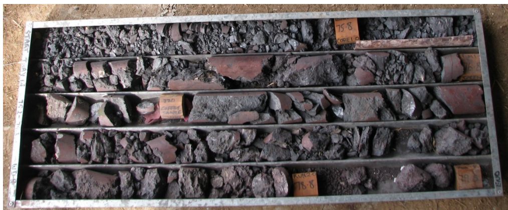
Figure: Example of iron ore drill core from the bulk sample sent for comminution test work.
