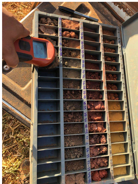
Figure 7: Enova's professional geologist is checking the magnetic susceptibility of saprolite drill cuttings during logging
