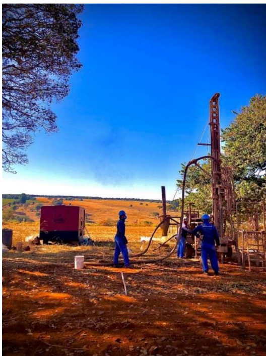
Figure 6: Reverse circulation drill rig in the backdrop of vast pastureland of CODA North.
