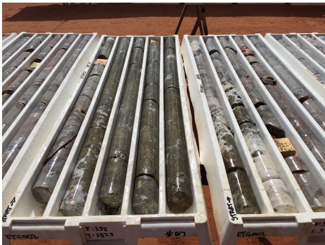
Photo 1: Eastern margin of stockwork corridor mineralisation at the Egg Prospect, Telfer West ETG0002 ~330m to 342m downhole core width ~50mm
