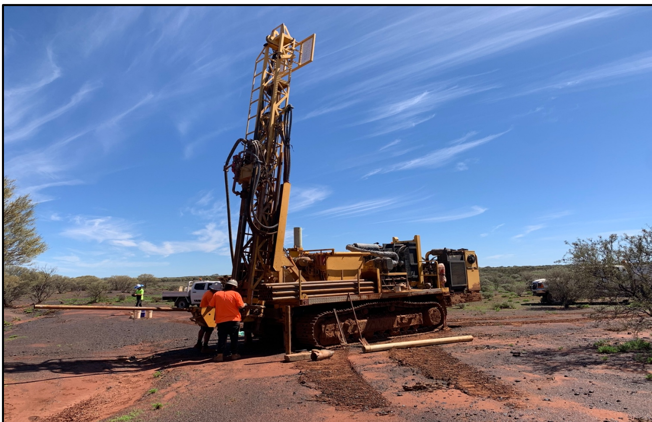
Figure 1 - RC drill rig set up at Weelarrana Manganese Project
