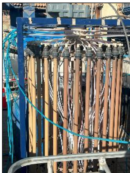
Figure 13-12: Cobalt Loading onto BPA Resin
