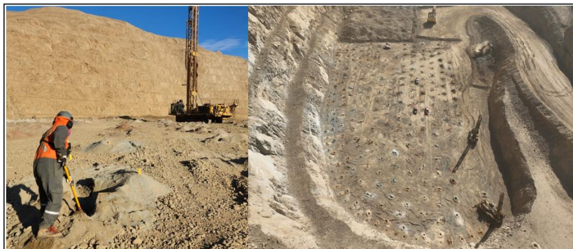
Figure 11-3: Blast Hole Drilling and Sampling
