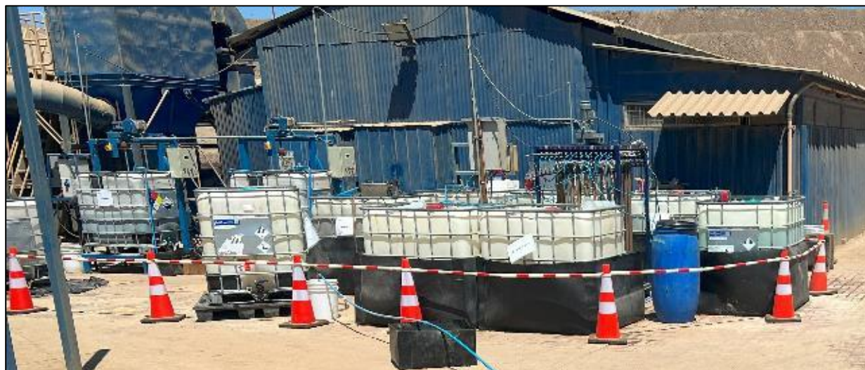
Figure 13-11: Pilot Ion Exchange Circuit at Mantoverde for The Recovery of Synthetic Cobalt Solutions
