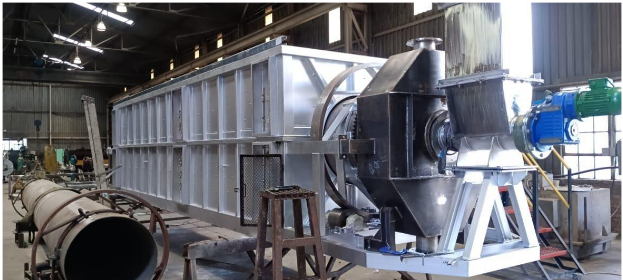
Figure 4: Calciner at Kayelekera is mechanically complete
