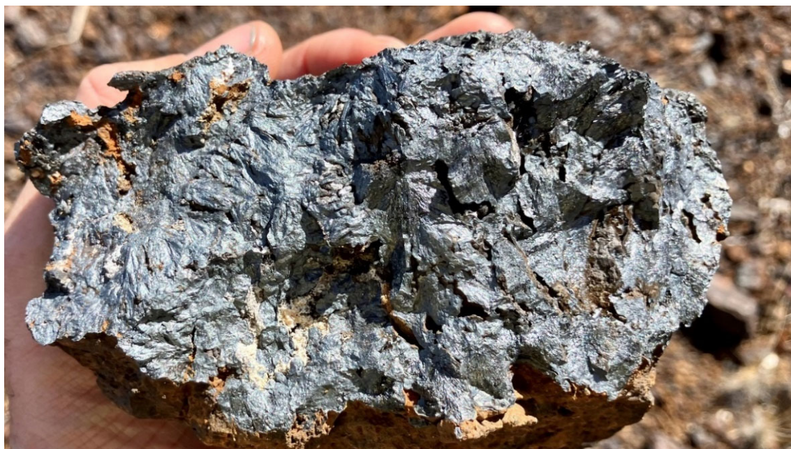
Figure 9. Manganite sample showing pyrolusite needles (Sample#ZEU110).
