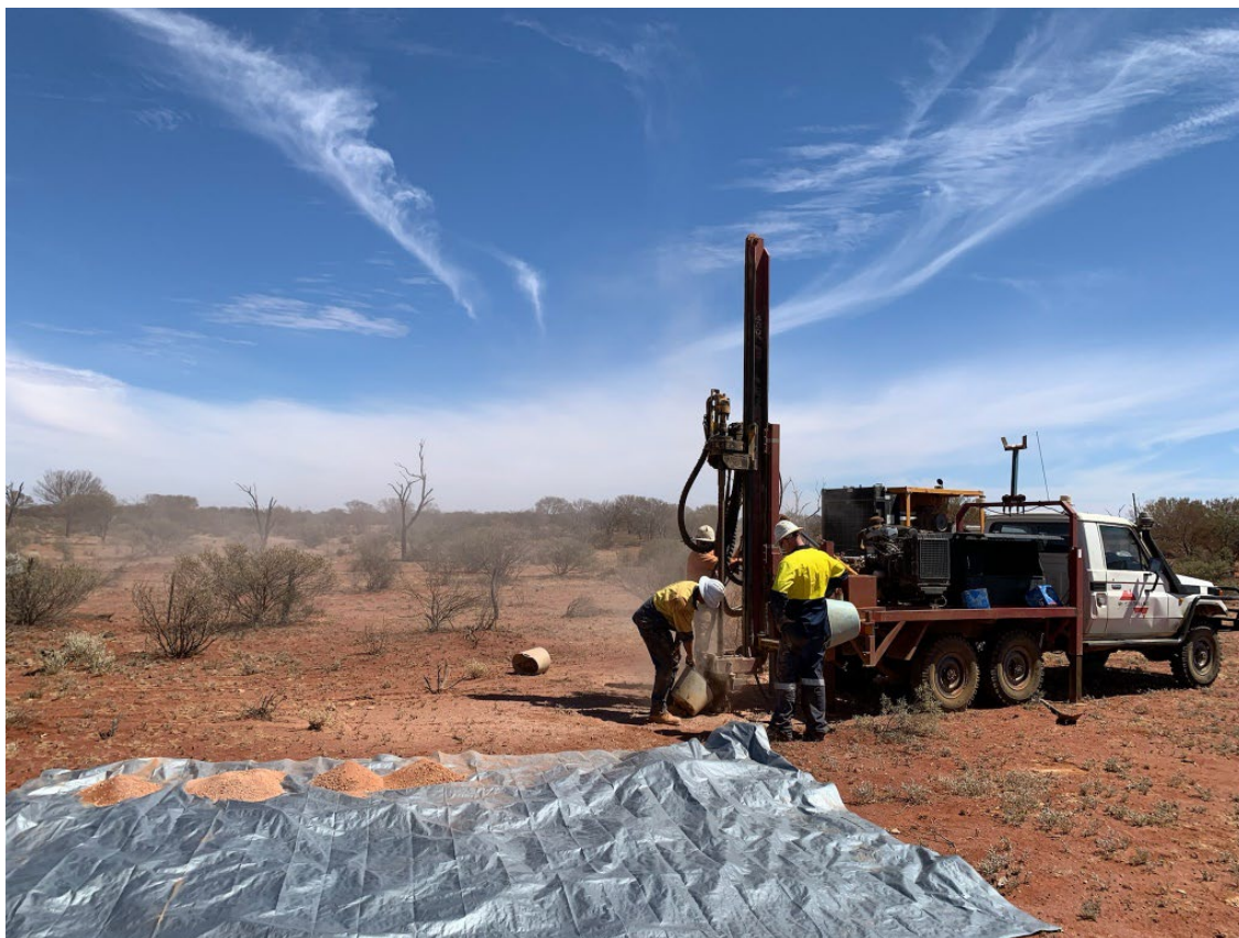
Photo RAB Drilling Operations at Comet
