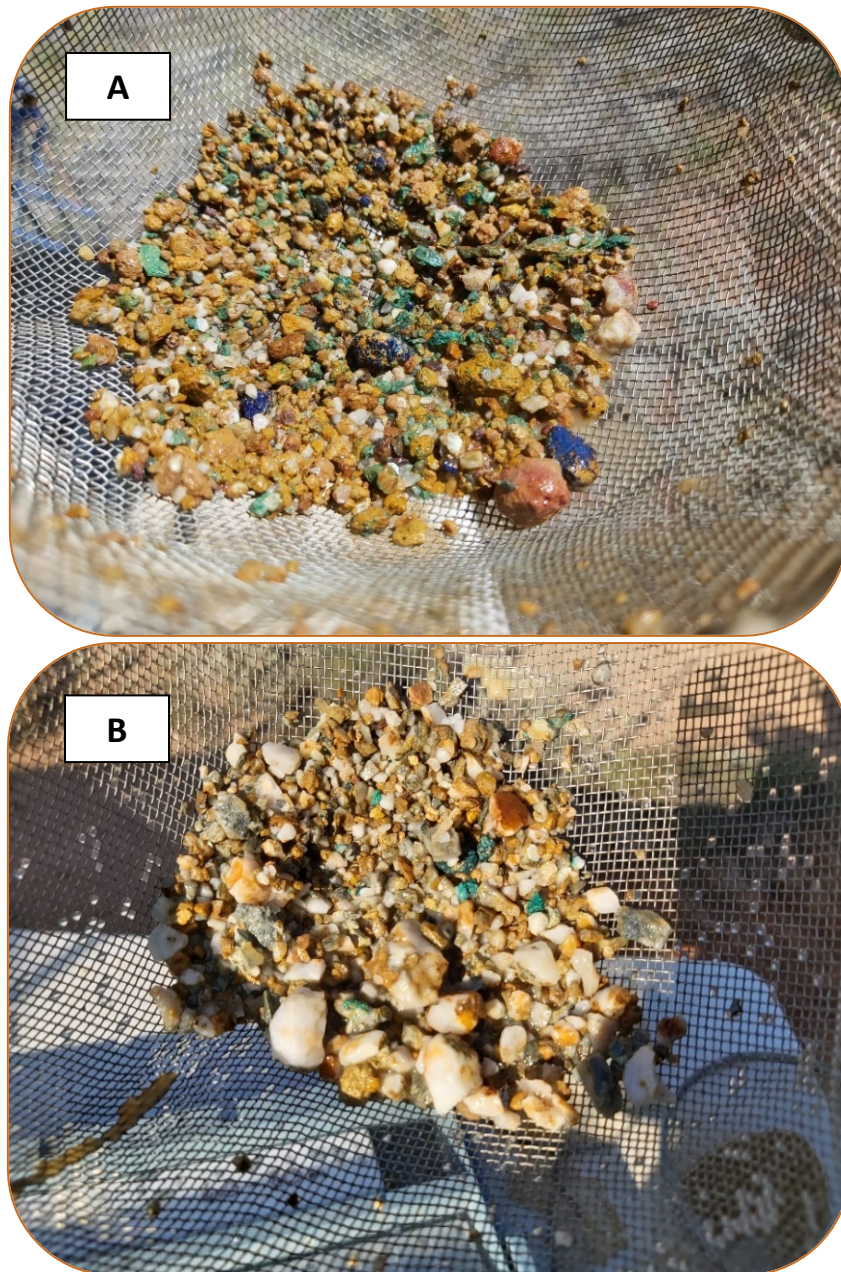
Figure 8 – Copper oxide mineralisation. A: malachite, azurite and quartz in CORC0141 at 38m. B: malachite and quartz in CORC0144 at 39m.
