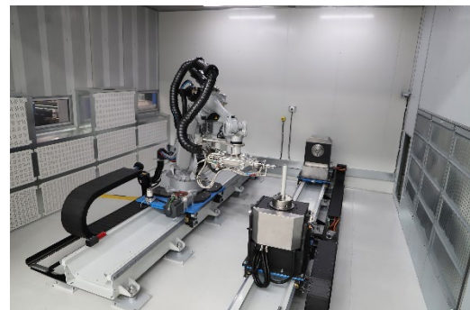
Figure 3 Titomic TKF 3250 in Melbourne, Australia – capable of large, seamless part manufacturing.
