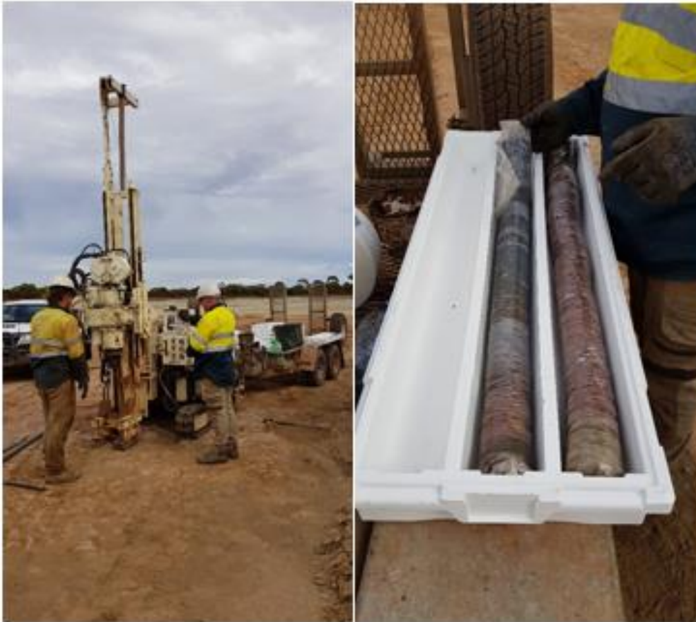
Figure 13 - Sonic rig drilling on SST dam (left) and example of sonic 'core' (right)
