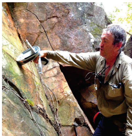
Figure 6: Analysing veins at the Birdwood project using a portable analyser
