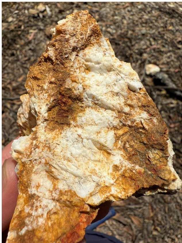
Figure 2 – Gold mineralisation within ferruginous rusty quartz vein yielding 63.10g/t Au from sample 3001227
