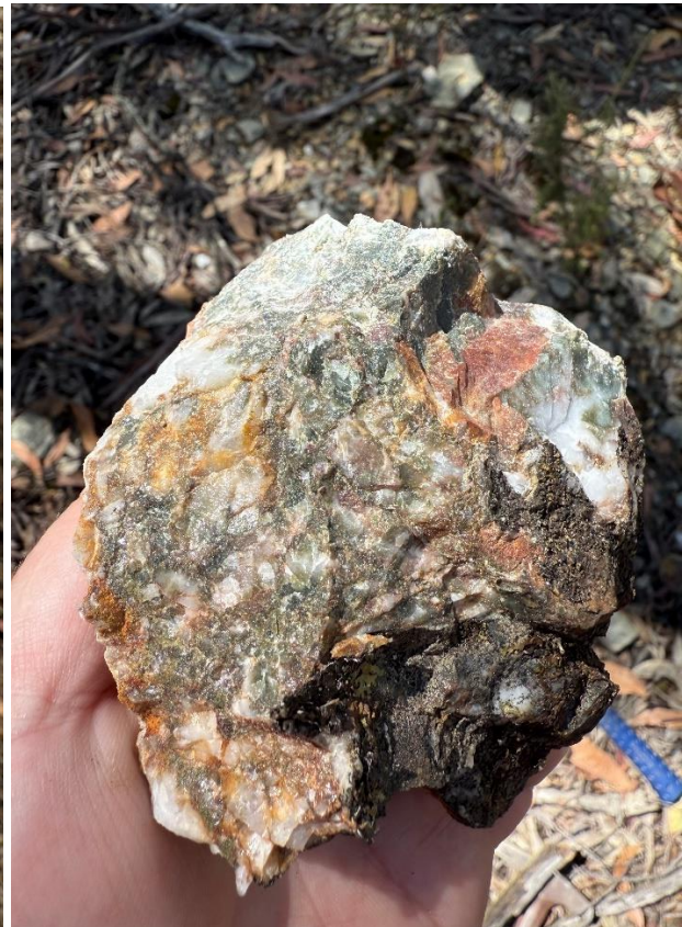
Figure 3 – Gold mineralisation within chloritic- quartz vein yielding 55.80 g/t Au from sample 3001131
