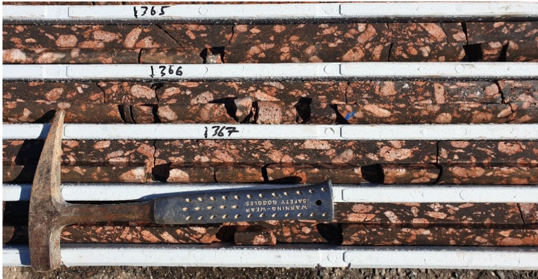
Photo 1 – Hole ID MCDA5-01 – Photo of core tray box 52, showing a portion of the igneous breccia sequence. The dark matrix comprises chlorite-clay-hematite altered igneous rock. Clasts comprise coarse K-feldspar from the local host granite. The matrix is enriched in the light rare earths, cerium, and lanthanum.
