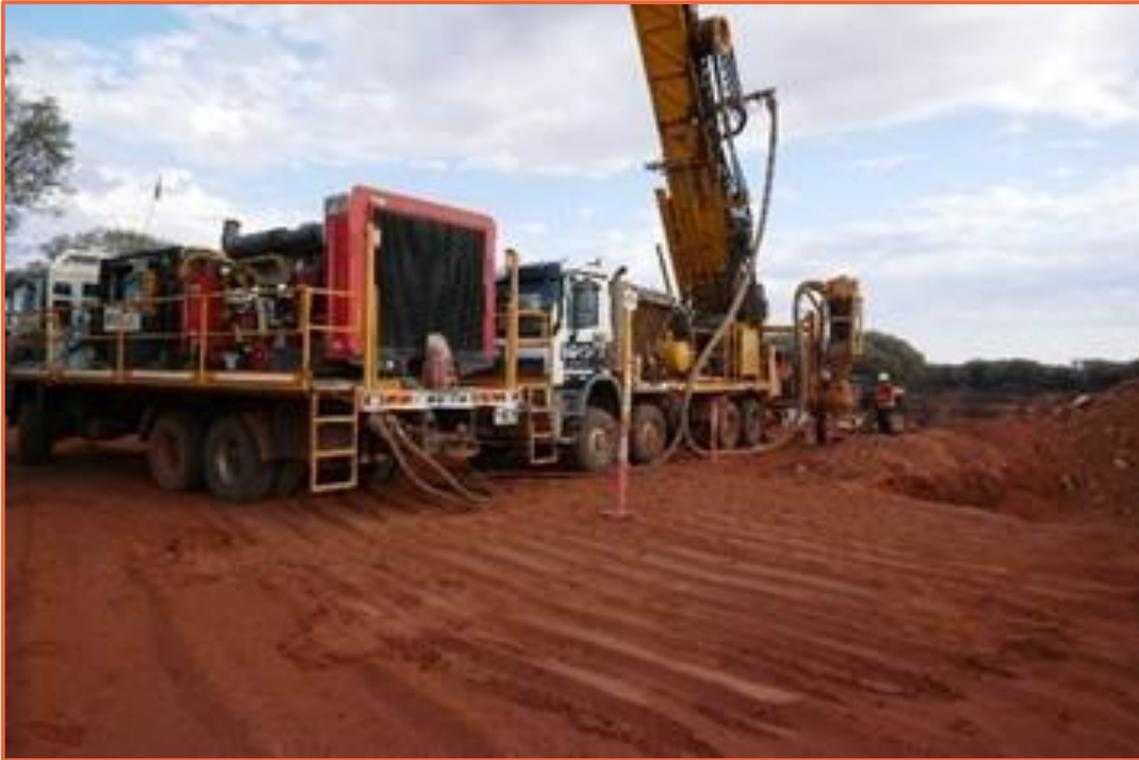
Figure 4 – Example of RC Drill Rig in Operation as part of delivering the Stage 10 Programme.
