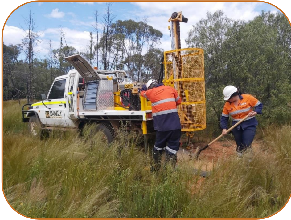
Figure 8: Auger Rig in action on Helix's tenements
