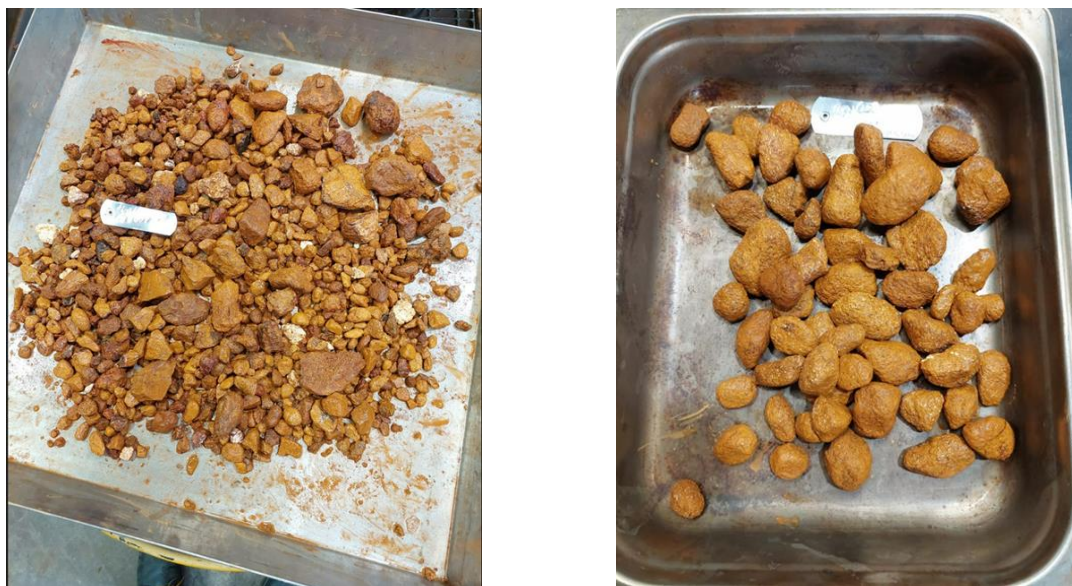
Figure 23. Batch Scrubbing of ore after 8 minutes. Left photo shows discharge after scrubbing and right side shows agglomerates after hand sorting (larger agglomerates are around 50 mm in diameter).
