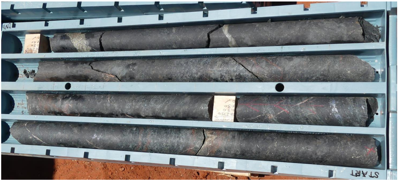
Figure 13: 21MHDD002 (272.2 – 275.7m) – massive magnetite skarn with disseminated scheelite and molybdenite (metallic silver) mineralisation and bands of chalcopyrite (yellow).
