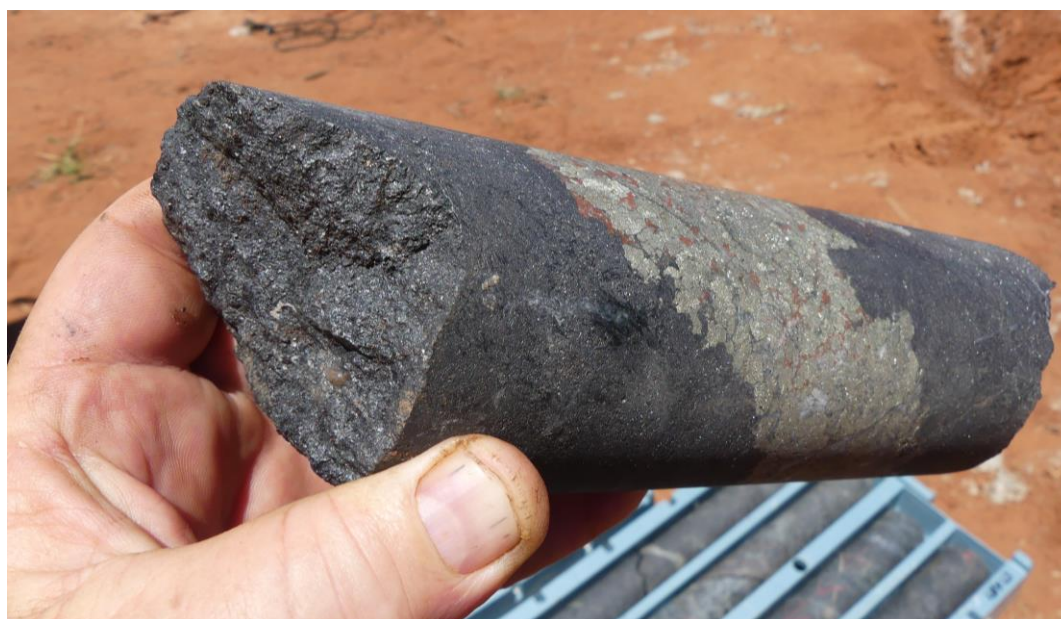
21MHDD002 (275.4m) -massive magnetite skarn with disseminated scheelite-molybdenite-chalcopyrite
