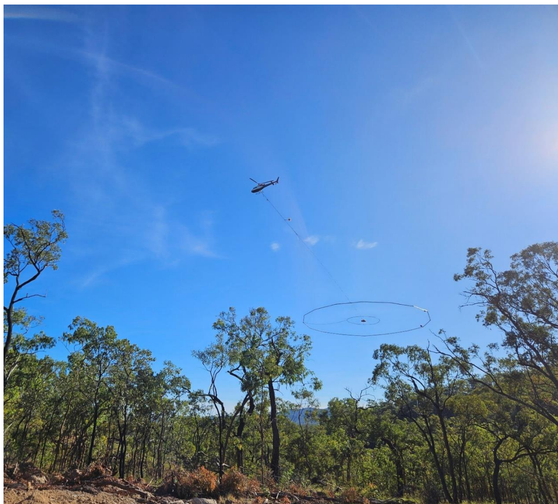
Figure 1 Helicopter borne VTEM Survey underway at Orient Silver-Indium Project
