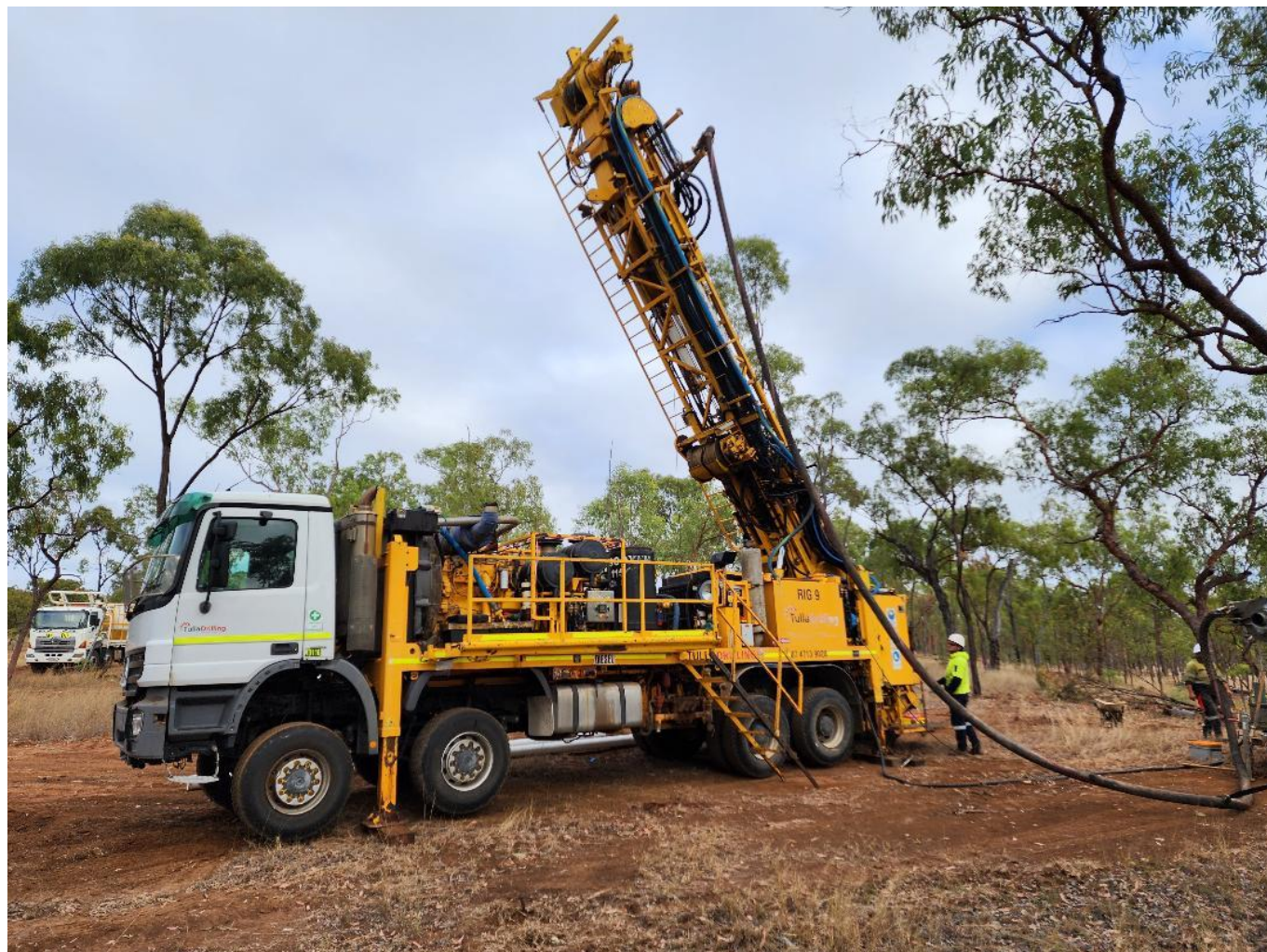
Figure 1: The multi-purpose DE840 rig currently drilling onsite.
