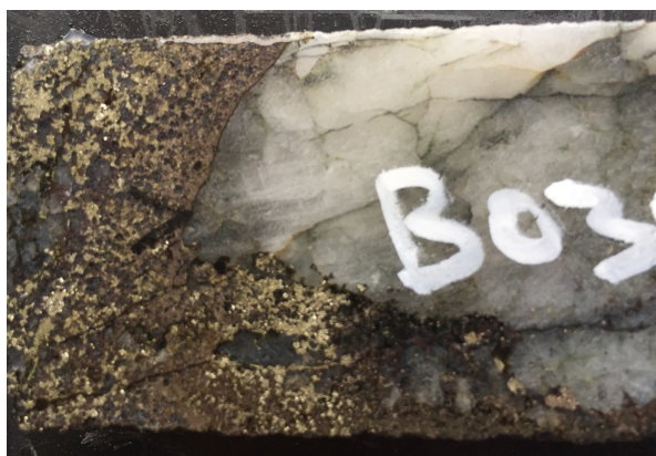
Figure 5: Late stage pegmatitic quartz vein with entrained sulphides derived from earlier VMS deposit displacing VMS mineralisation in this interval.
