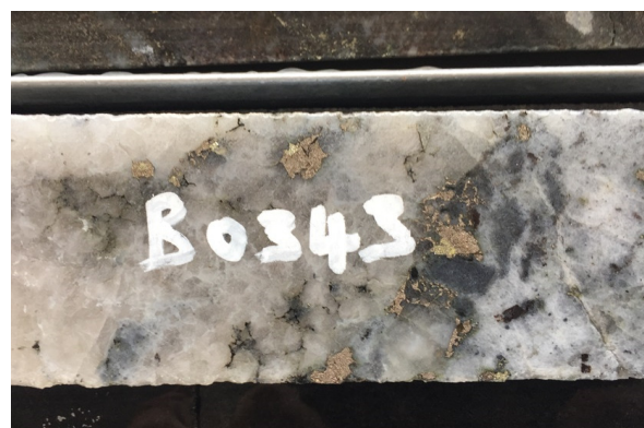
Figure 5: Late stage pegmatitic quartz vein with entrained sulphides derived from earlier VMS deposit displacing VMS mineralisation in this interval.
