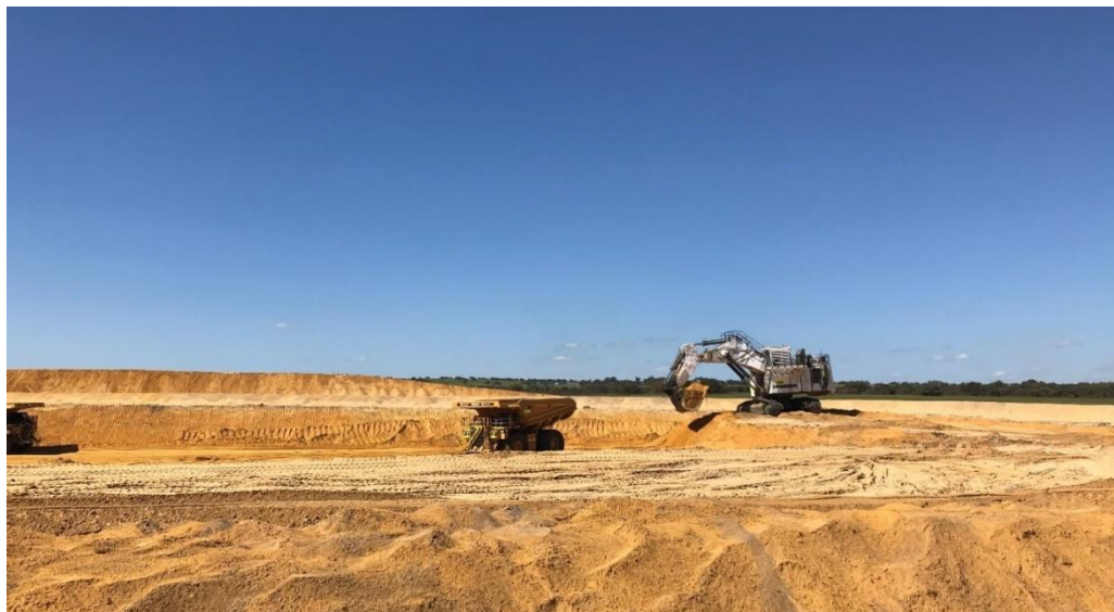
Figure 6 – Example of Overburden Mining
