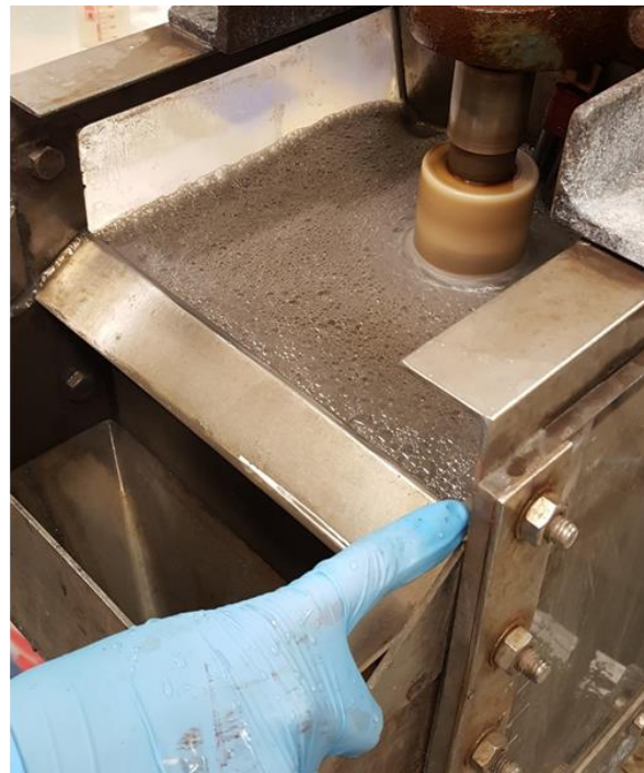
FIGURE 10: ZINC (Zn) ROUGHER-CLEANER FLOTATION TESTWORK – UP TO 58% Zn
