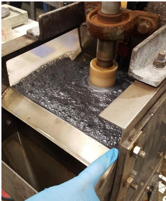
FIGURE 9: LEAD (Pb) ROUGHER-CLEANER FLOTATION TESTWORK – UP TO 79% Pb
