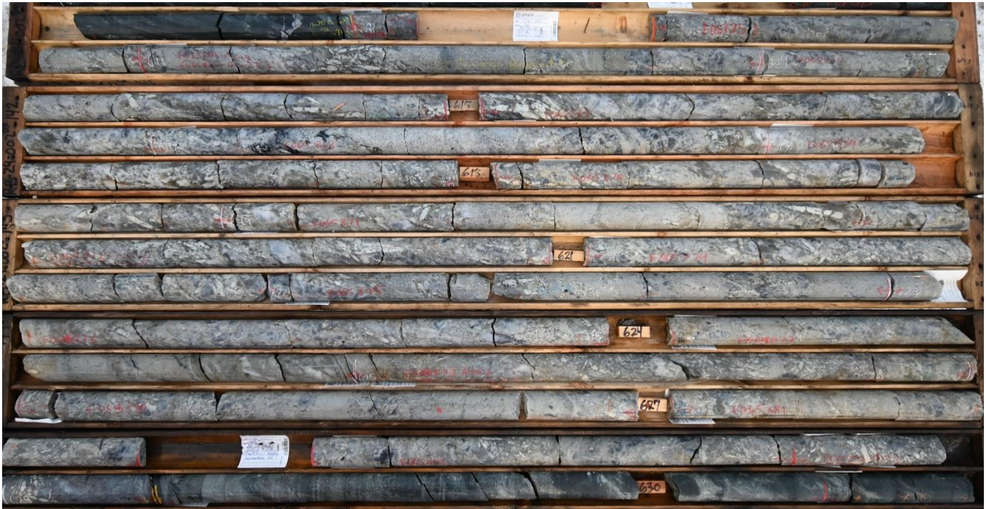
Figure 1: Pegmatite intercept 611.9-629.2m (RB-24-002: 17.3m @ 1.80% Li 2 O from 611.9m)
