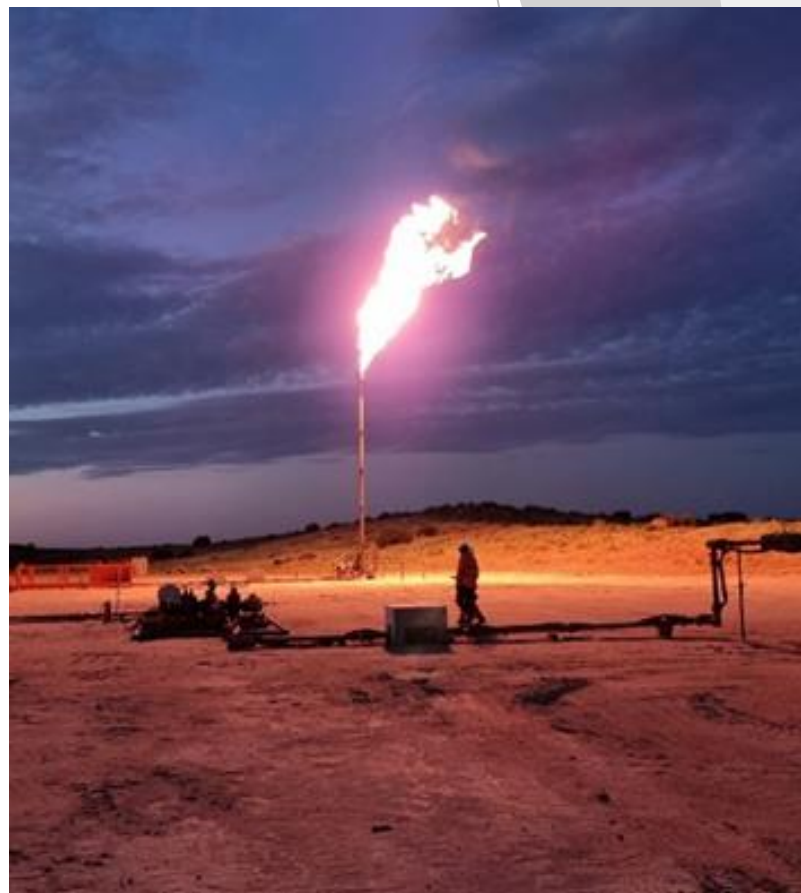
Figure 1: Gas flare from Kiwi-1 wellsite at 1.7 mmcfd
