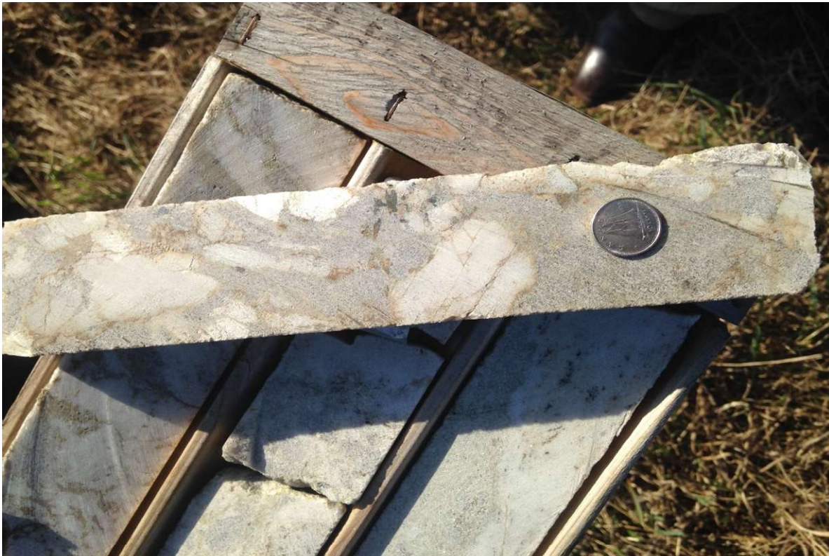
Figure 4: Spodumene crystals in drill core
