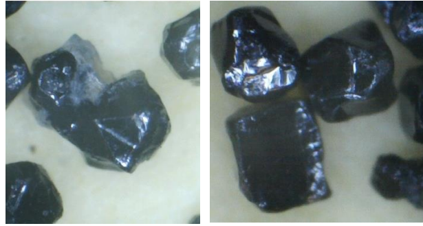
Figure 5. 300µm chromite ore particles: HSI product (left) and EDS mill product (right)
