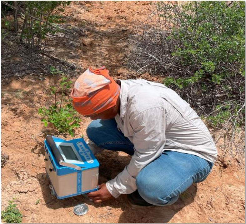
Undertaking gravity survey at NCP
