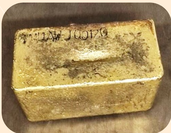
Figure 1. Doré bar at Three Mile Hill Mill
