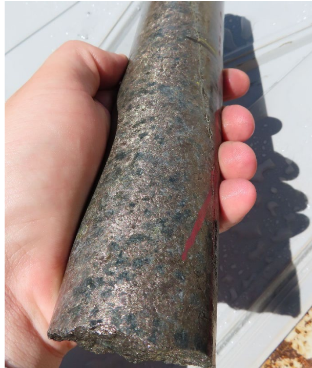
Photo 2: ANDD0015 drill core Semi-massive Ni-Cu sulphides @ 369.8-370.1m downhole
