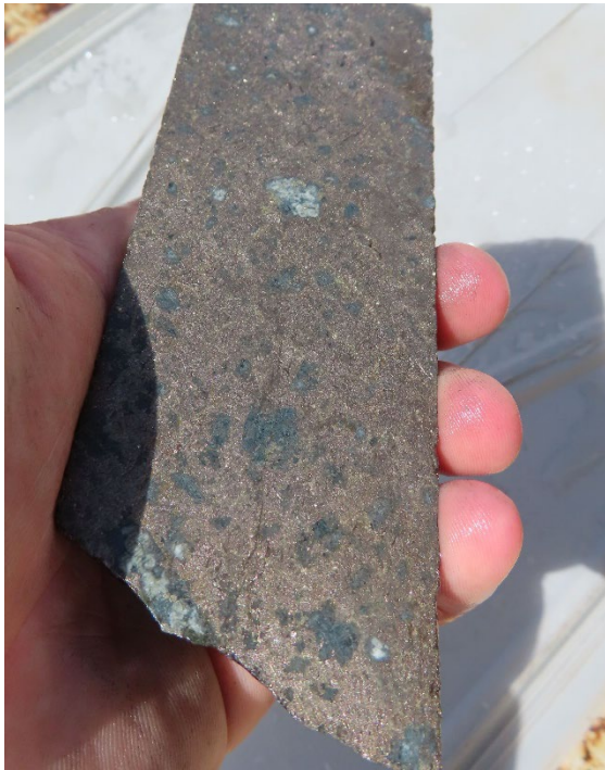
Photo 1: ANDD0014 drill core Massive Ni-Cu sulphides @ 456.1-456.3m downhole
