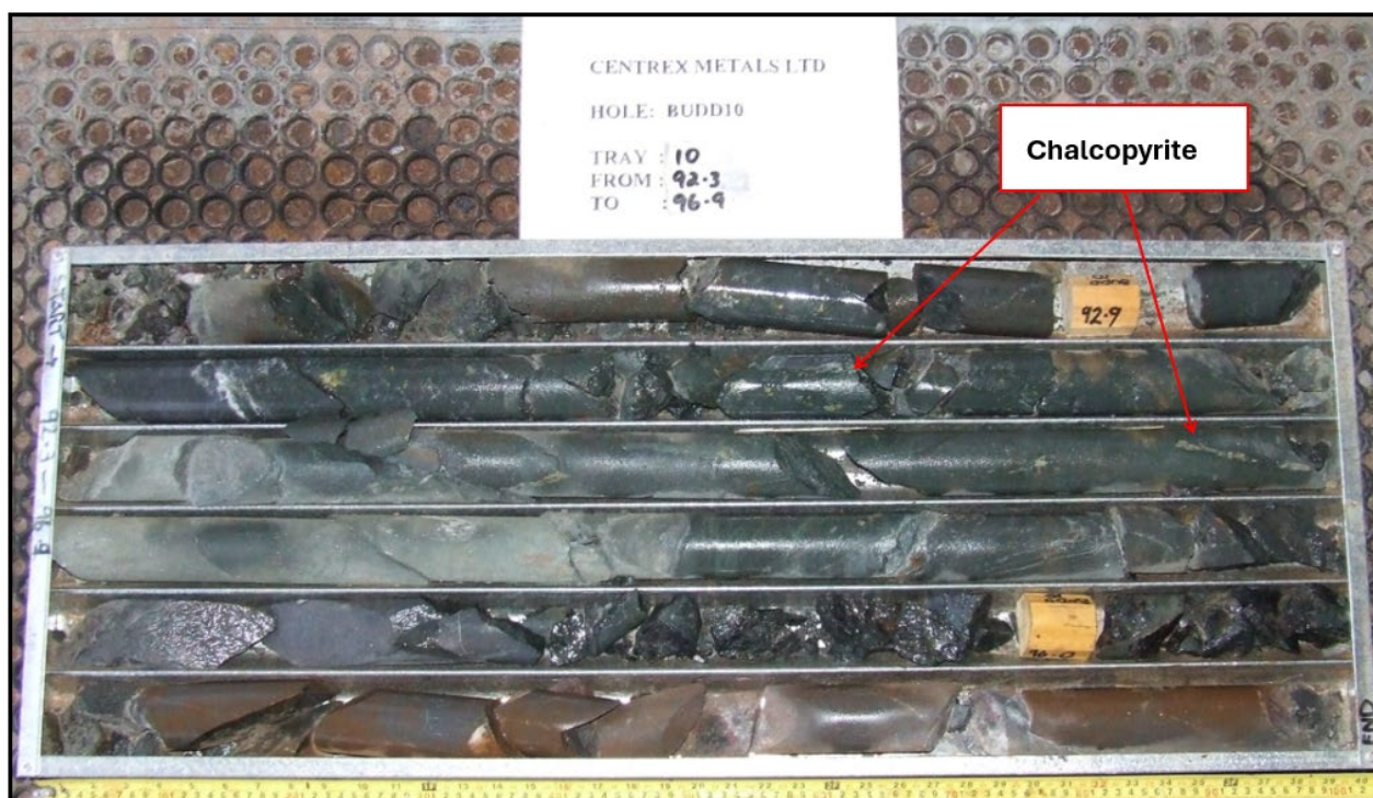
Figure 3. BUDD010 Core photo with visible chalcopyrite (Cu) mineralisation
