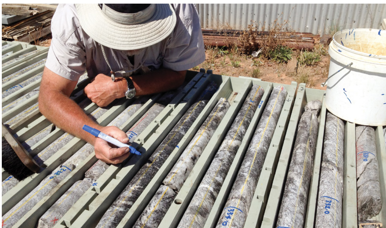
Thackaringa – Logging Diamond Drilling Cores
